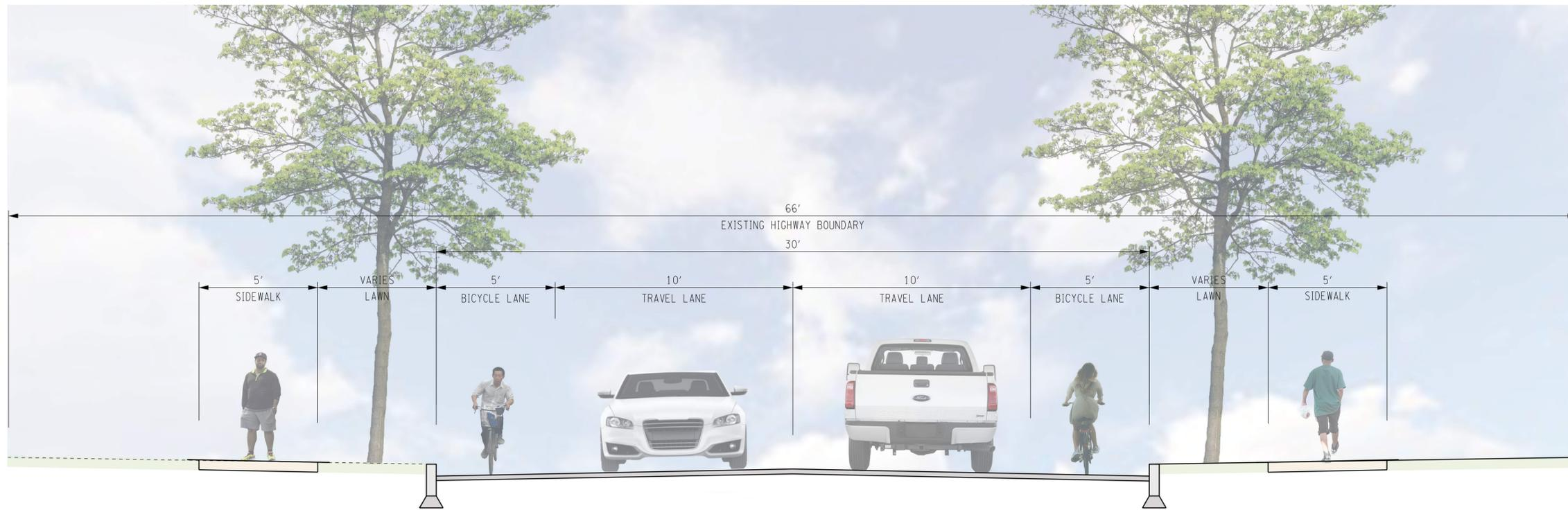
**CULVER ROAD - CONTINUOUS BIKE LANES, REMOVE LEFT TURN LANE AT SIGNALS
