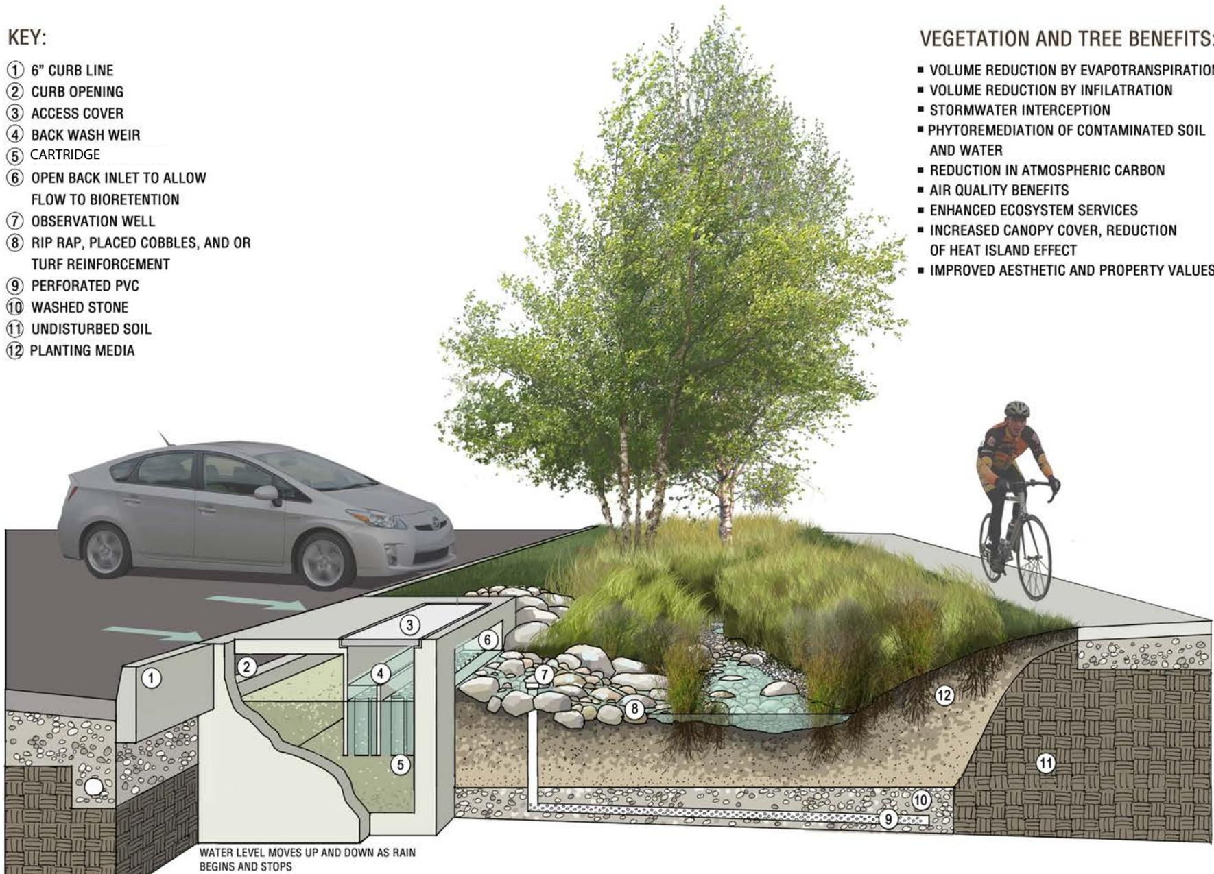
**BIORETENTION SYSTEM WITH PRETREATMENT CHAMBER**
