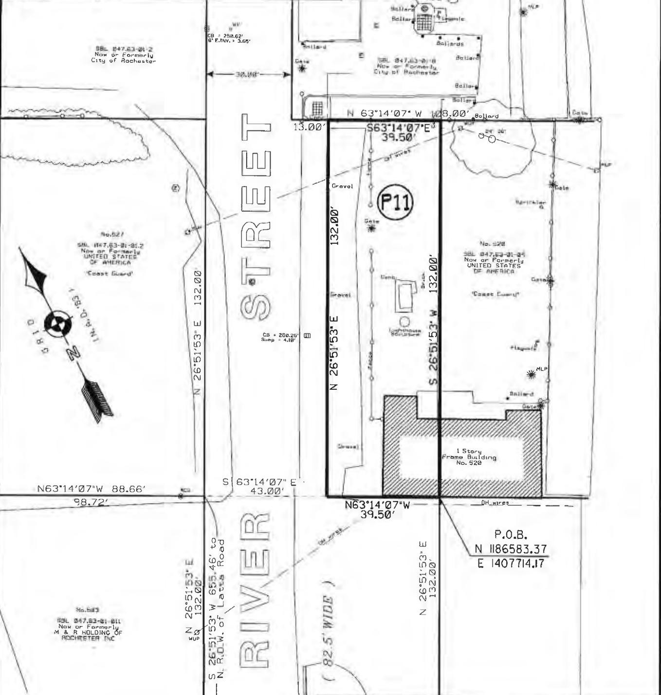
Coordinate pairs and bearings shown on this map were calculated through control ties to local geodetic control monuments in New York State Plane, Western Zone, NAD '83 feet.
