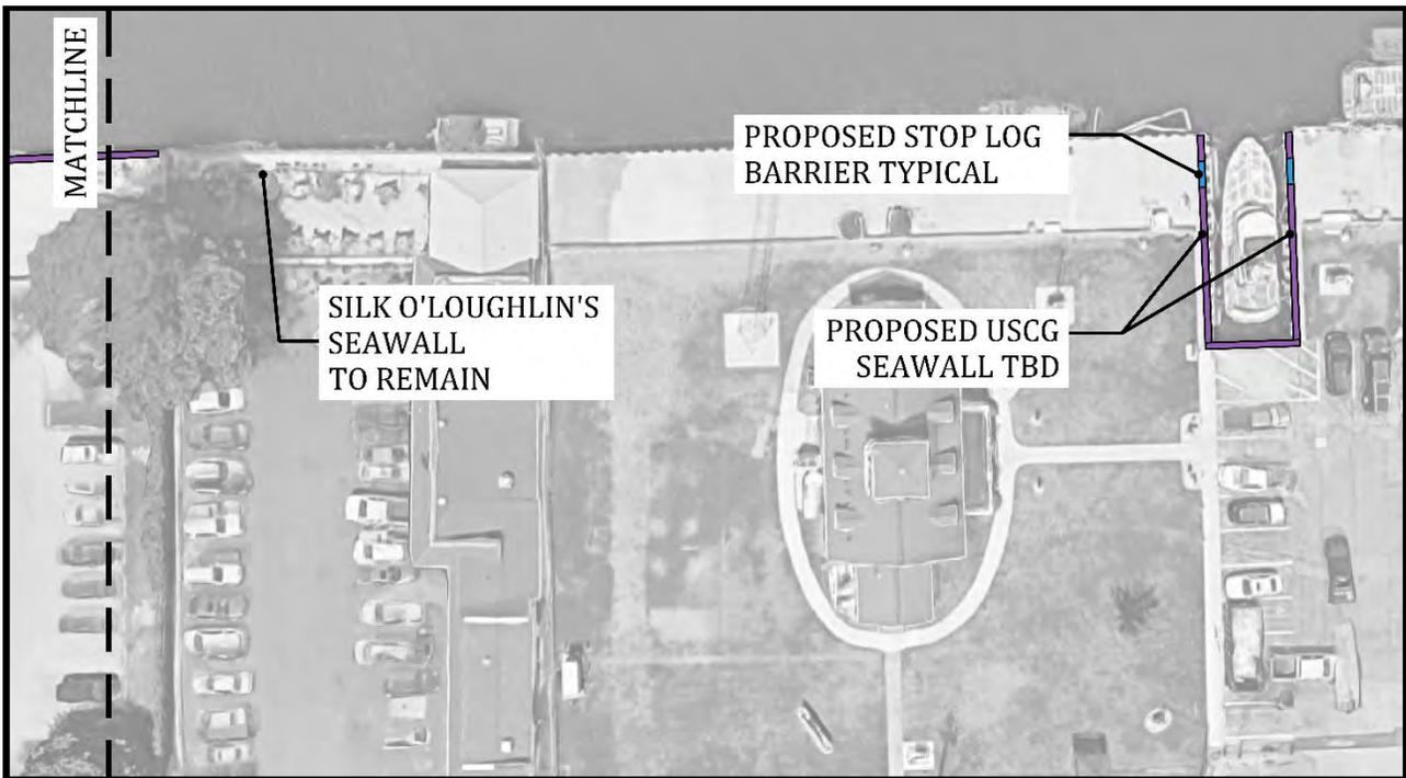
Figure 14 – Seawall Concept Plan C: Silk O'Loughlin's and USCG Station
