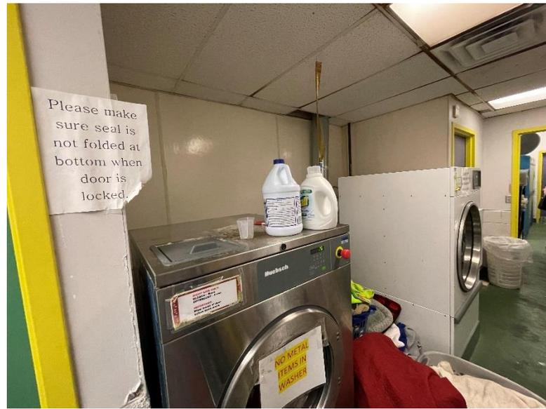
*The lack of a proper soiled hold has resulted in laundry baskets on the floor impeding the exit access.*
