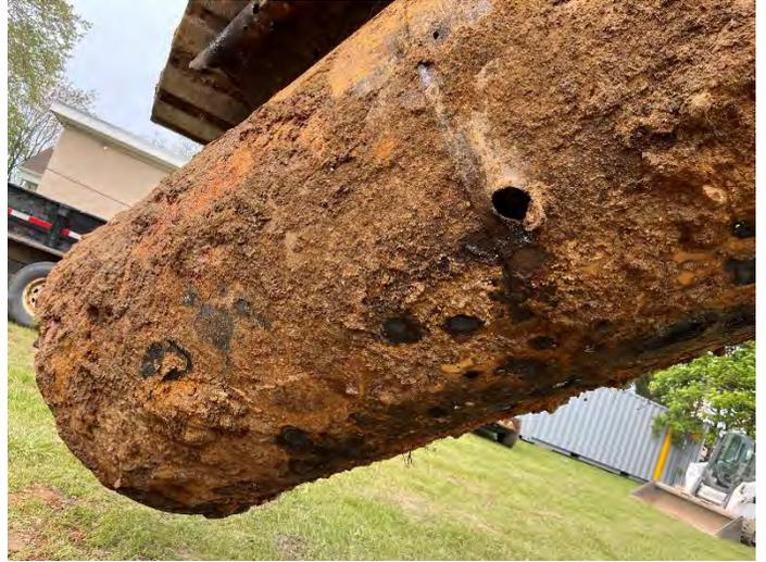
Photo No. 20 Apparent Geoprobe Hole on the Side of UST-03
