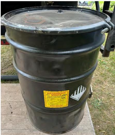
**Photo No. 35** Example Hazardous Waste Drum Labeling
