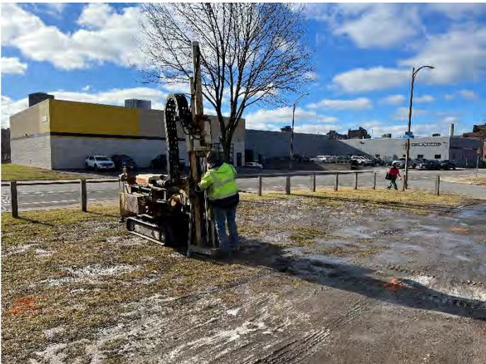
**Photo No. 3** Geoprobe Setup at GP-06
