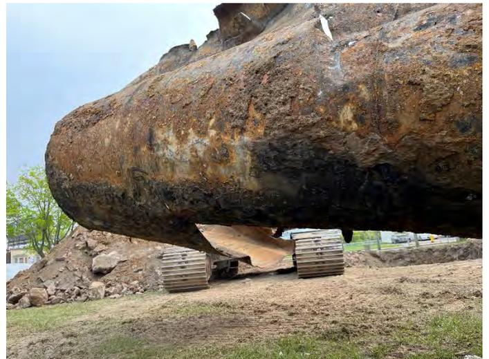
Photo No. 18 Bottom of UST-04 in Good Condition
