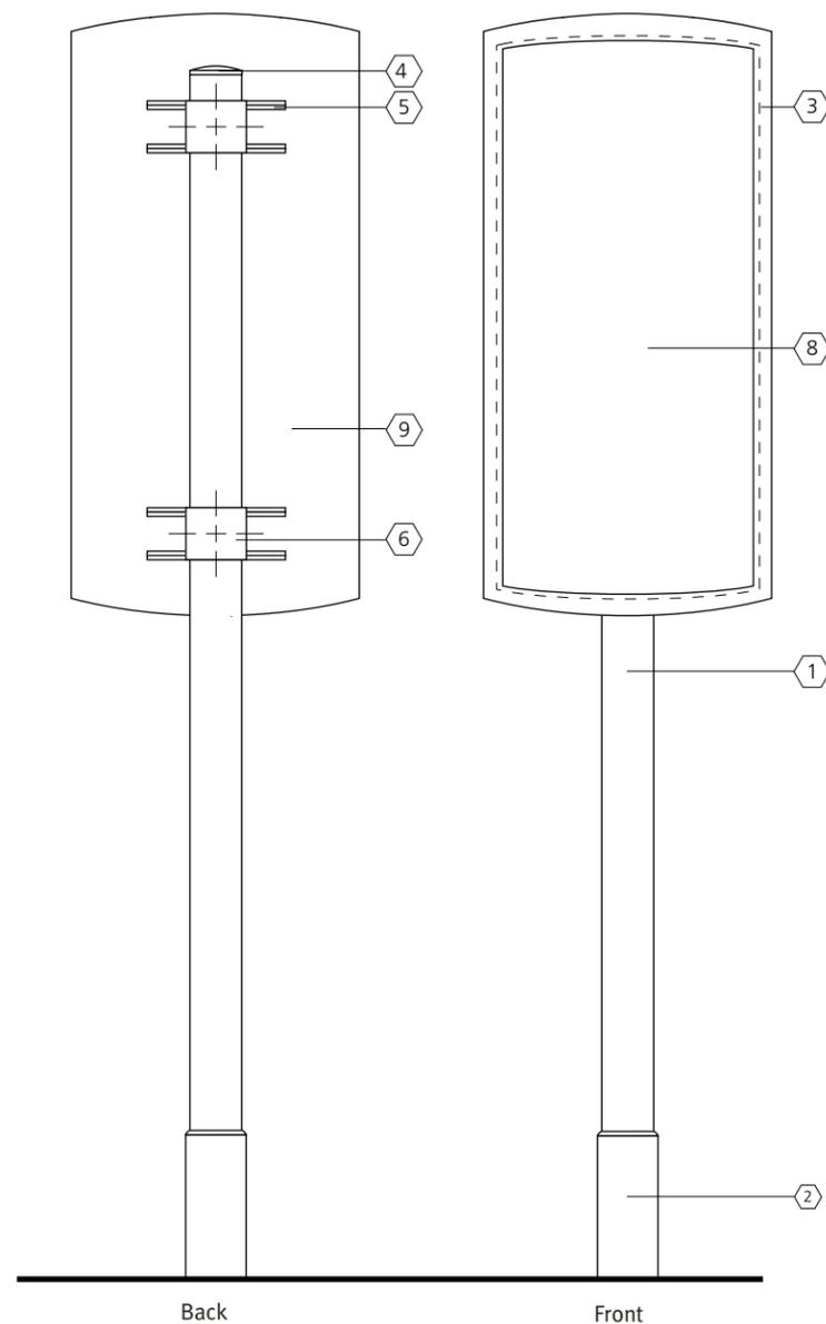
1 Typical detail for a single-faced minor kiosk
