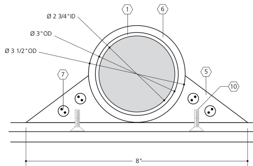
3 Typical construction & mounting details
