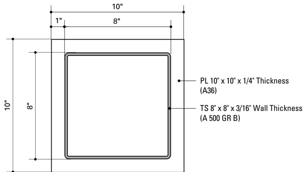
**3** Section View: Sleeve Foundation: Sleeve Detail
