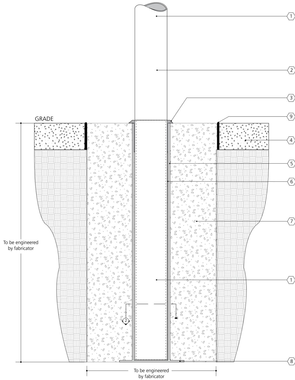
**1** Section Concrete Sleeve Footer
