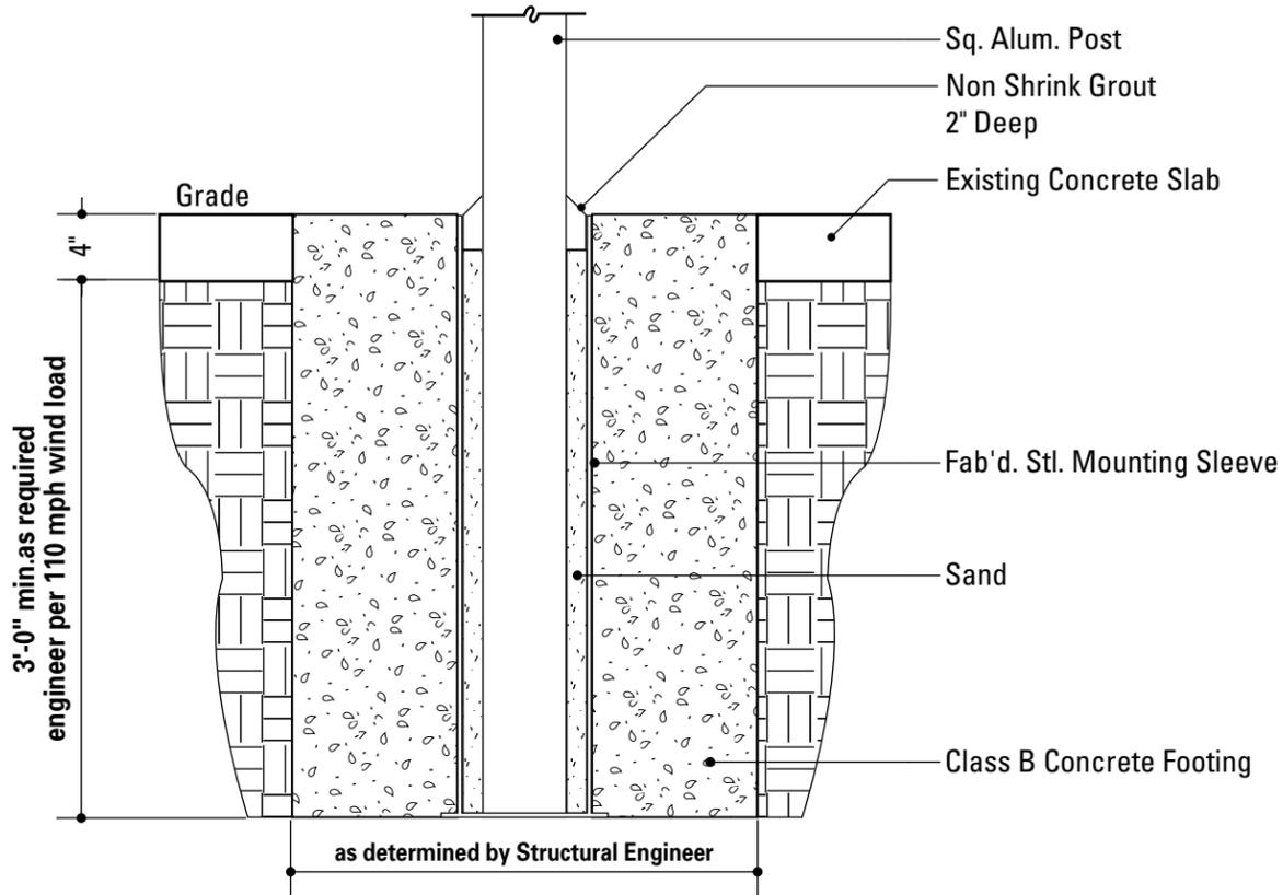
**1** Section View: Sleeve Foundation: Concrete
