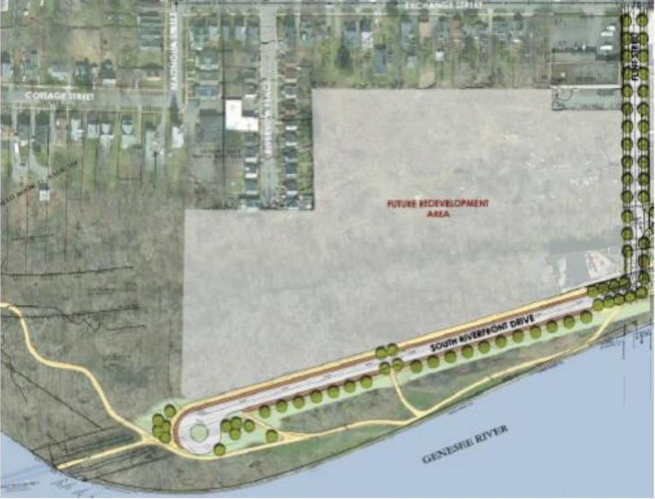
**Alternative 2:** Construction of a new waterfront street ending in a cul-de-sac
