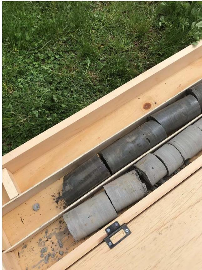
Monitoring Well MW-04 Rock Core with Sheen (5/9/2019)
