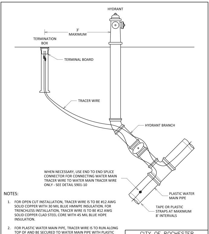
STRAPS OR TAPE PLACED AT MAXIMUM 8 FEET INTERVALS. AT WATER VALVE, TRACER WIRE IS TO RUN ALONG SIDE OF PLASTIC
