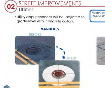
Note: Collars are only installed when an adjustment is necessary due to structural condition, frame & grate condition, elevation issues or for a new manhole or water valve.
