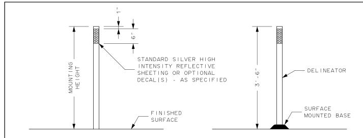
FLEXIBLE 21/4" DIAMETER YELLOW POLYETHYLENE PLASTIC TUBULAR POST WITH RECESSED CAP AND 13/4" INNER REINFORCEMENT TUBE
