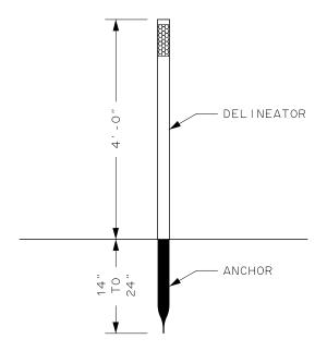
CLOSED-END DRIVE ABLE TUBULAR GALVANIZED METAL SOIL ANCHOR IN STANDARD LENGTHS OF 14",18" AND 24"
