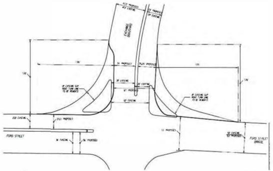
2. A decrease in pavement width of 7 feet, from 55 feet to 48 feet, beginning approximately 68 feet south of the Corn Hill Landing
