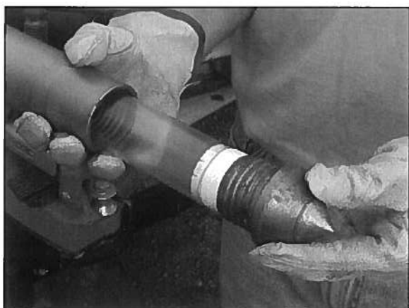
Figure 4.20. Slide whole assembly into either end of the sample tube.
