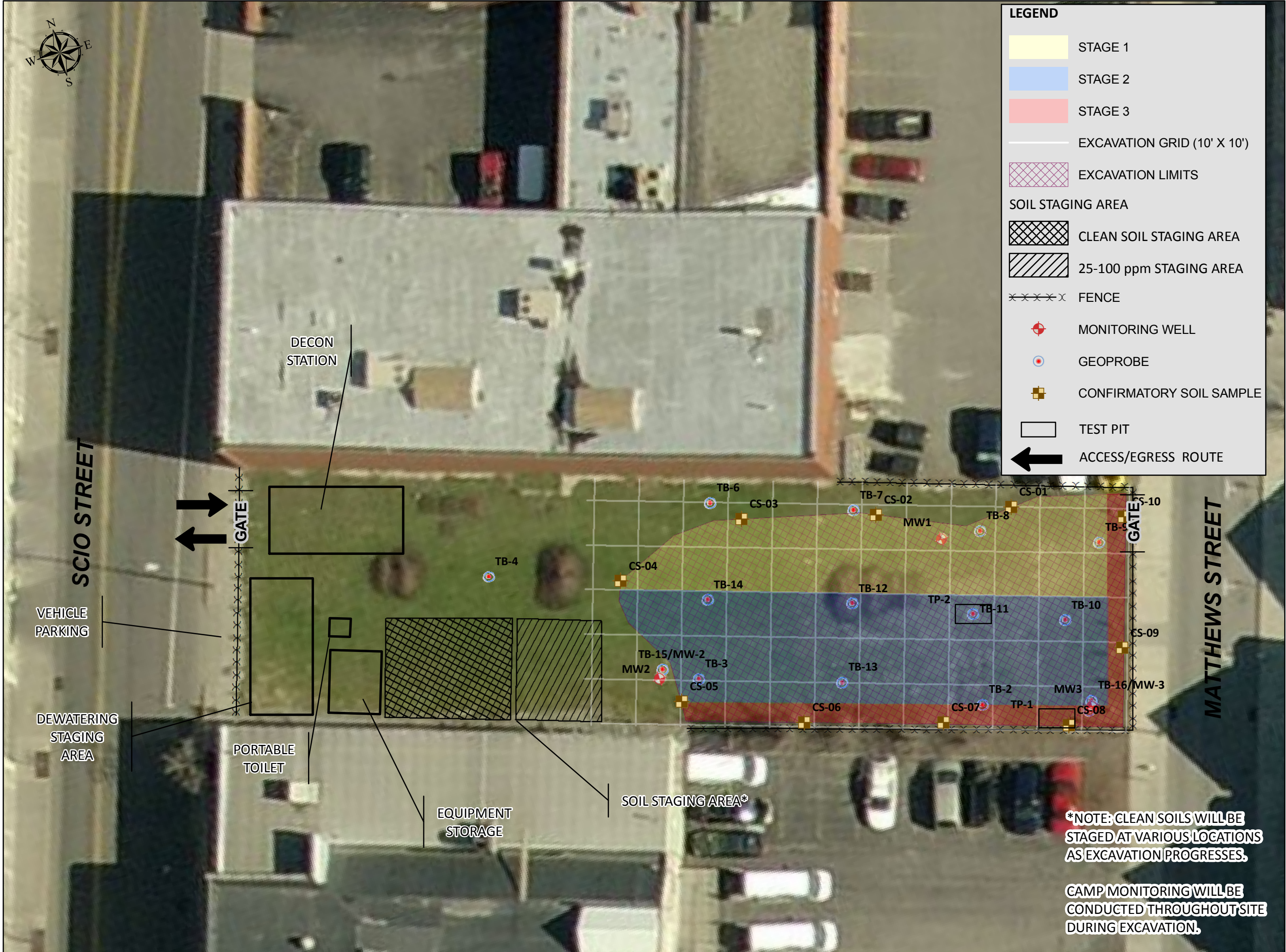
FIGURE 3 SITE LAYOUT AND EXCAVATION SEQUENCING
