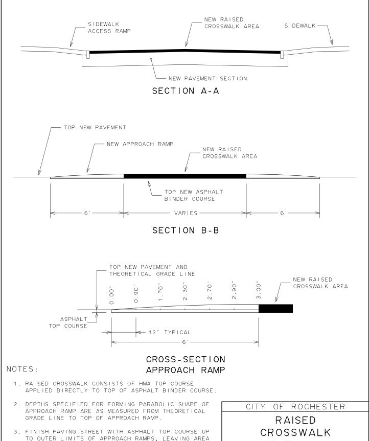
4. CLEAN PAVEMENT SURFACE, APPLY TACK COAT AND TREAT ALL EDGES WITH ASPHALT PAVEMENT JOINT ADHESIVE BEFORE CONSTRUCTING RAISED CROSSWALK.
