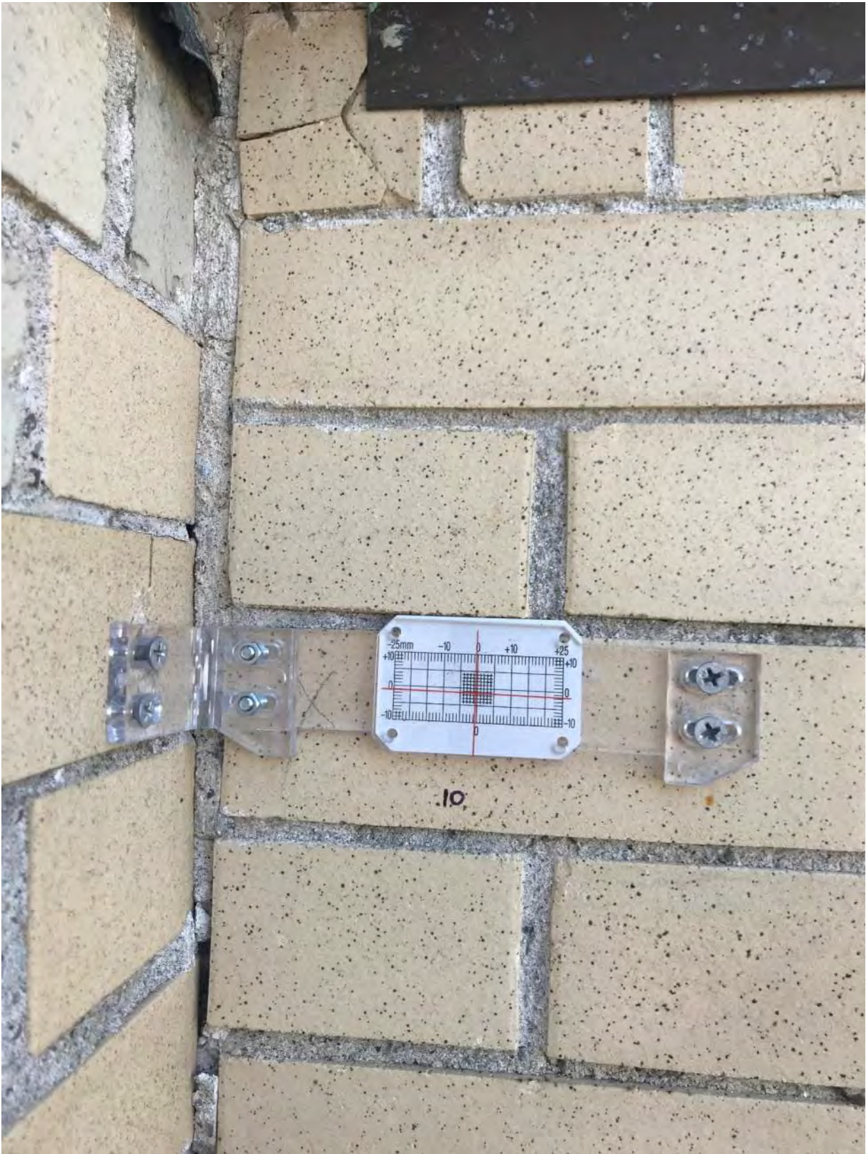
-0.5 mm Horizontal Movement | 1.5 mm Vertical Movement
