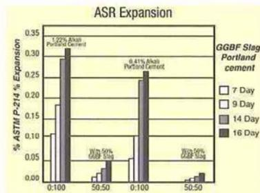
ASR Expansion. Reduced alkali-silica reaction
