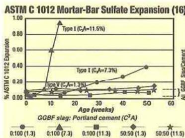
ASTM C1012 Mortar Bar Expansion: Improved sulfate resistance over Type V cement.
