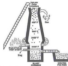
Iron and slag making process through a blast furnace.
