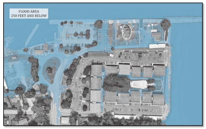
Figure 7: Flood Inundation Map for Lake Ontario Base Flood Elevation (250 Feet)
