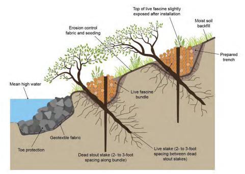
Figure 4-1 Vegetative Erosion Control/ Bank Stabilization
