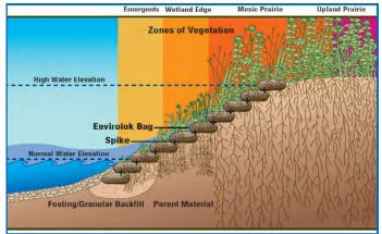
Figure 4-2 Envirolok Bank Stabilization Schematic (Source: Envirolok.com)
