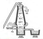
Iron and slag making process through a blast furnace.
