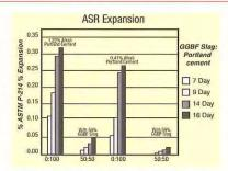
ASR Expansion. Reduced alkali-silica reaction
