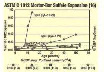
ASTM C1012 Mortar Bar Expansion: Improved sulfate resistance over Type V cement.
