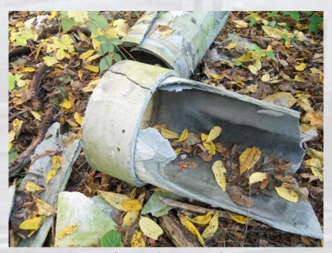
**Broken Vent Cap suspect ACM**
