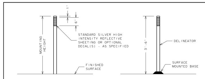
FLEXIBLE  $2\frac{1}{4}$ " DIAMETER YELLOW POLYETHYLENE PLASTIC TUBULAR POST WITH RECESSED CAP AND  $1\frac{3}{4}$ " INNER REINFORCEMENT TUBE
