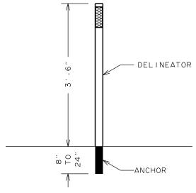
OPEN-END TUBULAR GALVANIZED METAL ANCHOR IN STANDARD LENGTHS OF 8", 14",18" AND 24"
